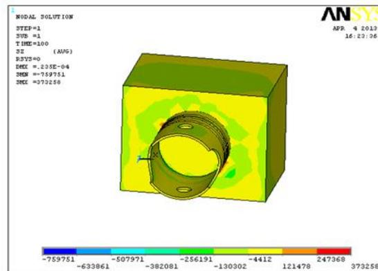
Fig. 10 Normal Stress distribution in Z axis
