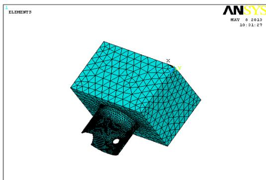
Fig. 4. Model mesh generation cylinder block and piston
