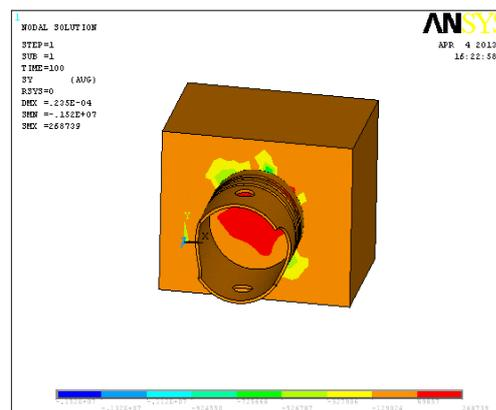
Fig. 9 Normal Stress distribution in Y axis
