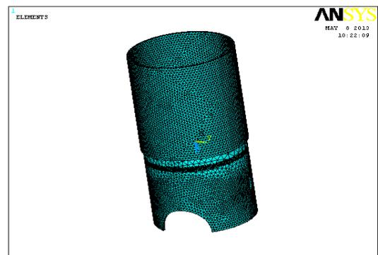
Fig. 5. Model mesh generation for cylinder liner and piston
