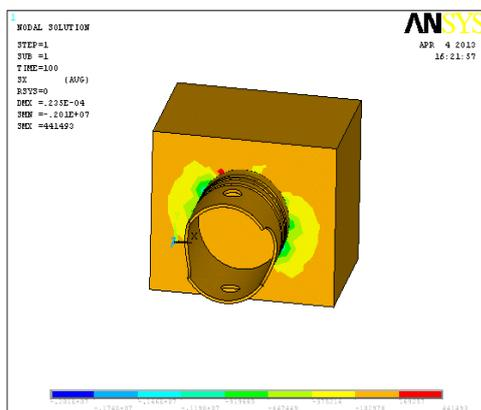
Fig. 8 Normal Stress distribution in X axis
