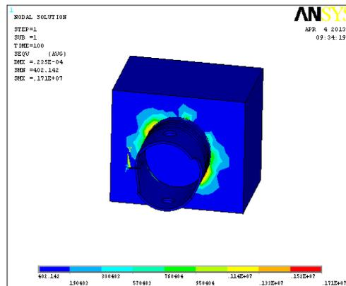
Fig. 7 Von-Mises Stress distribution
