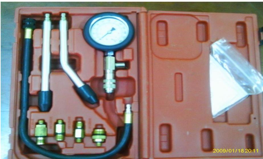
Fig.6 Gas cylinder compression tester
