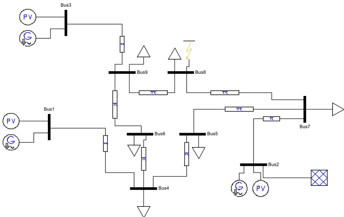
Figure 1: Power System model without energy storage
