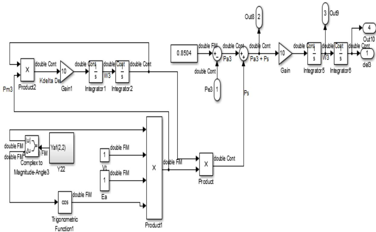
**Figure 6: A simulation diagram that compute power of the energy storage device,  $P_s$ , as function of time**
