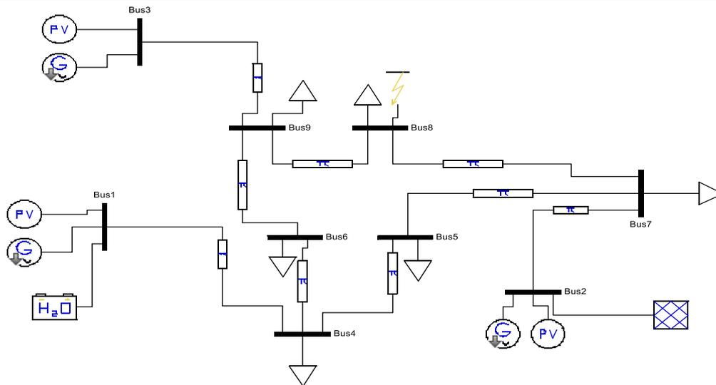
**Figure 2: Power System Model with Energy Storage Device**
