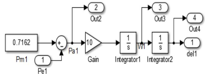
**Figure 4. : Simulation diagram for accelerating power and angular velocity of each generator rotor**
