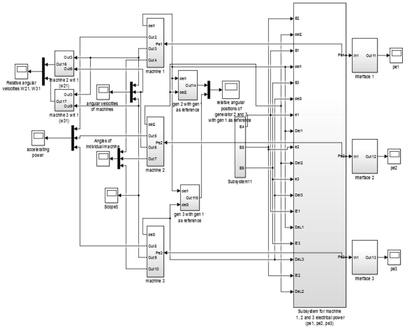
Figure 5: 9-Bus System used for transient stability analysis
