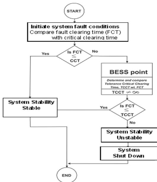
**Figure 3: Flowchart of the design with energy storage**
