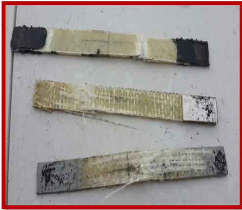
Fig. 12 photograph of failed specimens by tensile test.
