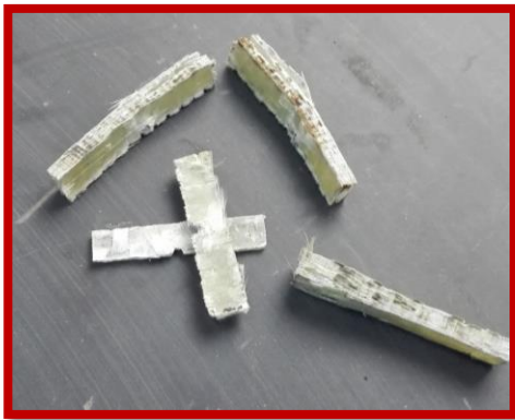
Fig. 13 photograph of failed specimens by impact test.
