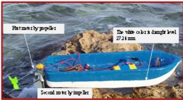
Fig.7 assembly the two small motor by brackets behind the boat.
