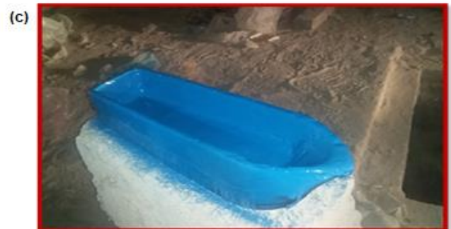
Fig.6 a the boat is lifted to cure at room temperature for 24 hours, b using silicon carbide paper to flatten the surface and remove rough edges, c color the boat by blue paint and white for draught level at 27.26mm.
