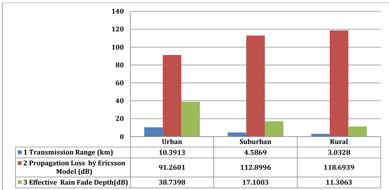
**Figure 2 Comparison of the simulation results for the three propagation environments; the urban, the suburban and the rural areas**
