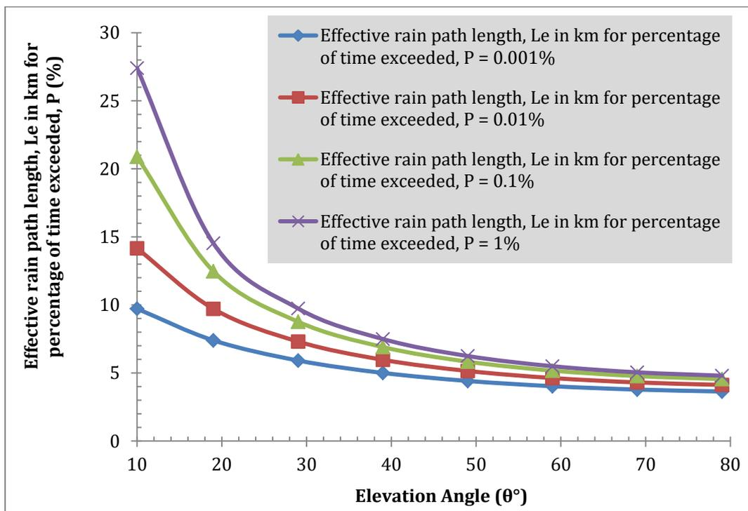
Figure 2 The results of effective rain path length,  $L_e$  in km for the selected percentage of time exceeded, P in the range of 1 % to 0.001%
