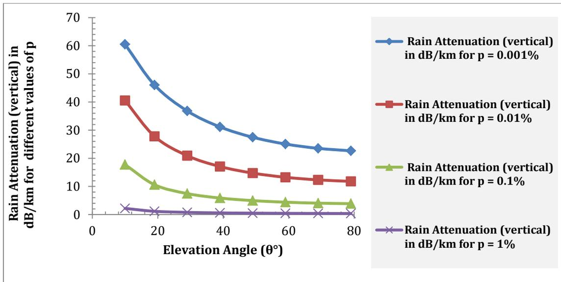
Figure 5 The results of rain attenuation in dB for the vertical polarization computed for various values of P and for the selected elevation angles
