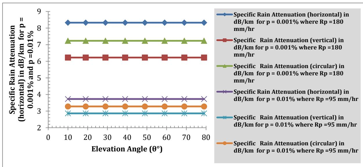
Figure 3 The results of specific rain attenuation in dB/km for  $p = 0.001\%$  where  $R_p = 180$  mm/hr and for  $p = 0.001\%$  and  $p = 0.01\%$  for the selected elevation angles
