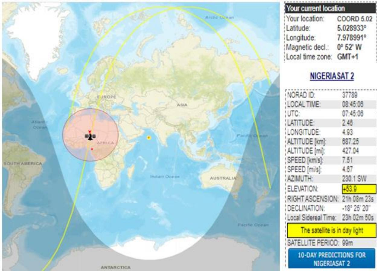
Figure 1 Map showing the NIGERIASAT 2 10-Day Tracking Predictions Data by n2yo.com where the orbit track is indicated by the yellow line, the satellite footprint is indicated by the transparent pink circle and the earth observation location is indicated by the red dot.
