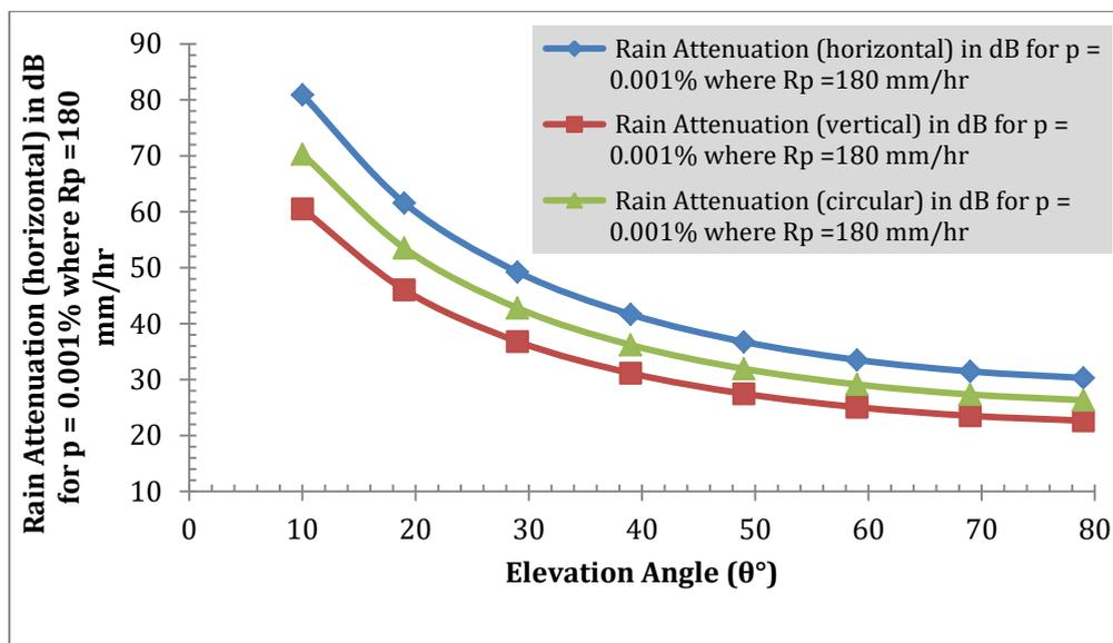
Figure 4 The results of rain attenuation in dB for  $p = 0.001\%$  where  $R_p = 180$  mm/hr for the selected elevation angles
