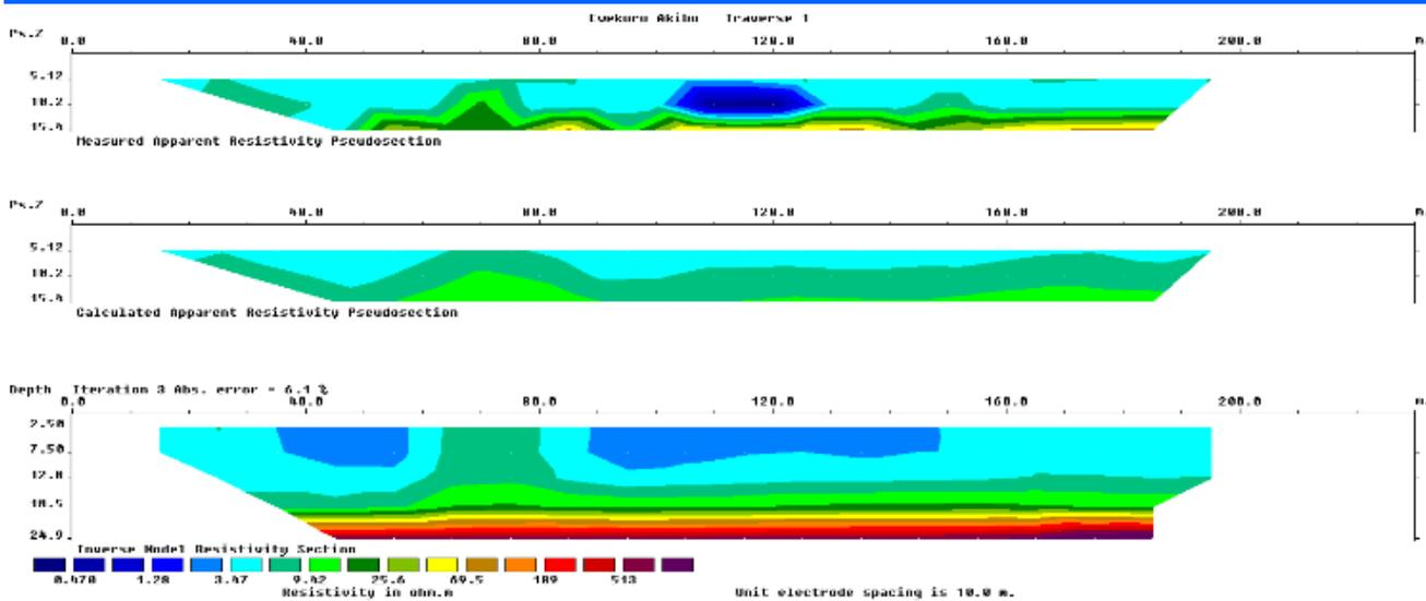
**Figure 4: Typical 2D-ERT inverse model along Ewekoro (Profile 1 and 2)**
