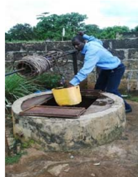
Fig. 2 Reeled bailer on tripod and pulley system
