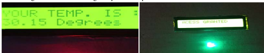
Figure 11 Picture showing the system's response when the participant's temperature falls within the allowable temperature set by the system
