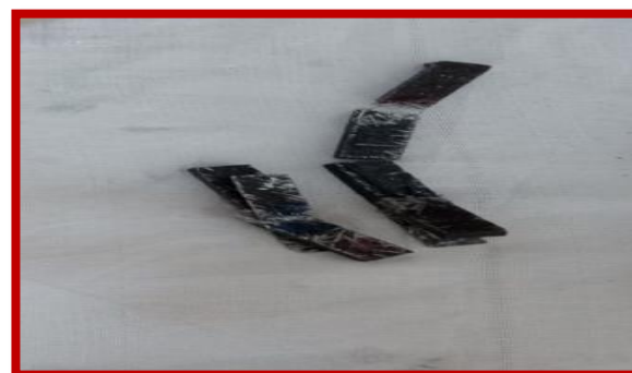
Fig. 15 photograph of failed specimens by impact test.
