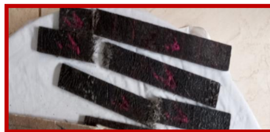
Fig. 14 photograph of failed specimens by tensile test.
